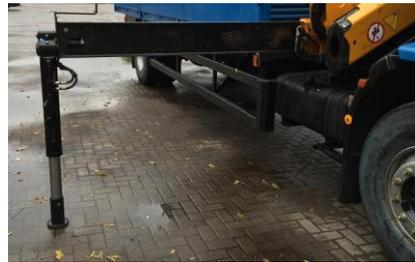
**Examples of Lorry Loader with partial deployment of Stabilizers (short rigging):**
