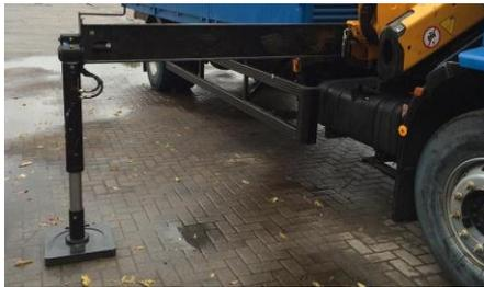
**Example of stabilizer fully deployed but without use of spreader pad:**
